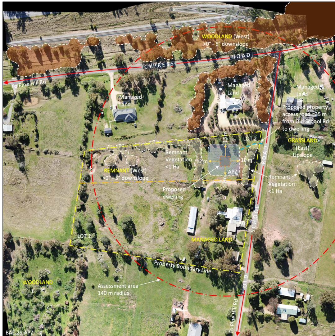
Figure 9 – Showing proposed BAL 29 APZ setback distances, vegetation classification, slope and property access for Lot 2. Indicative only. Not to scale. (Hague, 2023)
