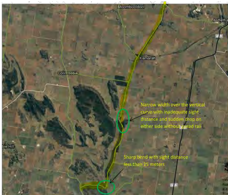
Fig 6: Gazettal of Kamrah Road for road train despite serious geometric and pavement width issues
